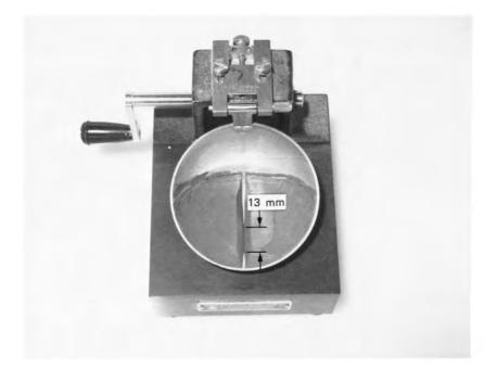
FIG. 8 Soil Pat After Groove Has Closed
