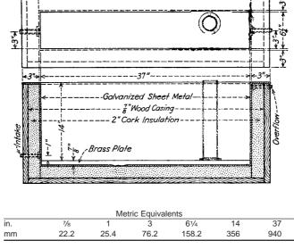
FIG. 4 Insulated Water Bath
