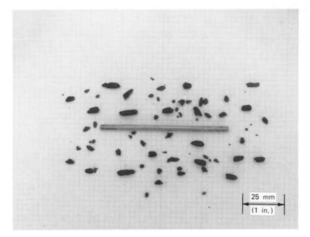
FIG. 9 Lean Clay Soil at the Plastic Limit
