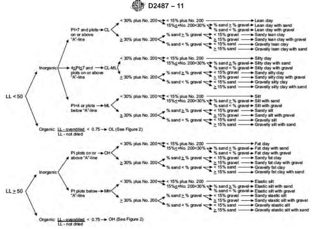
FIG. 1 Flow Chart for Classifying Fine-Grained Soil (50 % or More Passes No. 200 Sieve)
