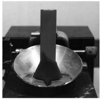
FIG. 6 Example of Grooving Tool Placed in a Properly Grooved Soil Pat
