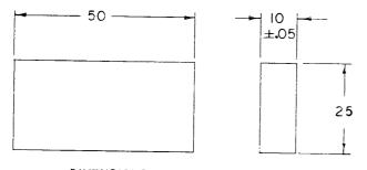
DIMENSIONS IN MILLIMETRES FIG. 4 Height-of-Drop Gauge
