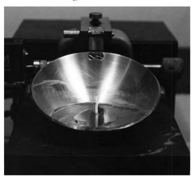
FIG. 7 Grooved Soil Pat in Liquid Limit Device
