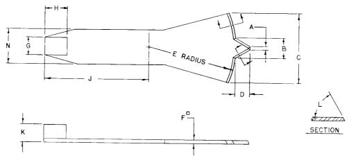
FIG. 3 Grooving Tool (Optional Height-of-Drop Gauge Attached)
